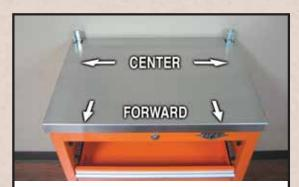
4. Set COUNTERTOP onto MAIN FRAME. Press down to COMPLETELY FLATTEN silicone. Slide COUNTERTOP FULLY FORWARD with equal overhang on sides. Use masking tape to hold COUNTERTOP while silicone dries.
